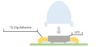
Ensure no floating or tilting of lens before curing Recommended for opaque or room temp-curing adhesives
