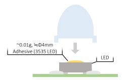
Ensure no floating or tilting of lens before curing
